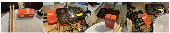
Please secure the two hi-hat cables in place with the cable clip, (included) while leaving some slack in the cables. If not, the cables could start jumping and create false triggering or may interfere with the chick sound.
